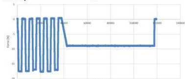
Figure 1 – Example of a load against sample graph from a sensitivity test
