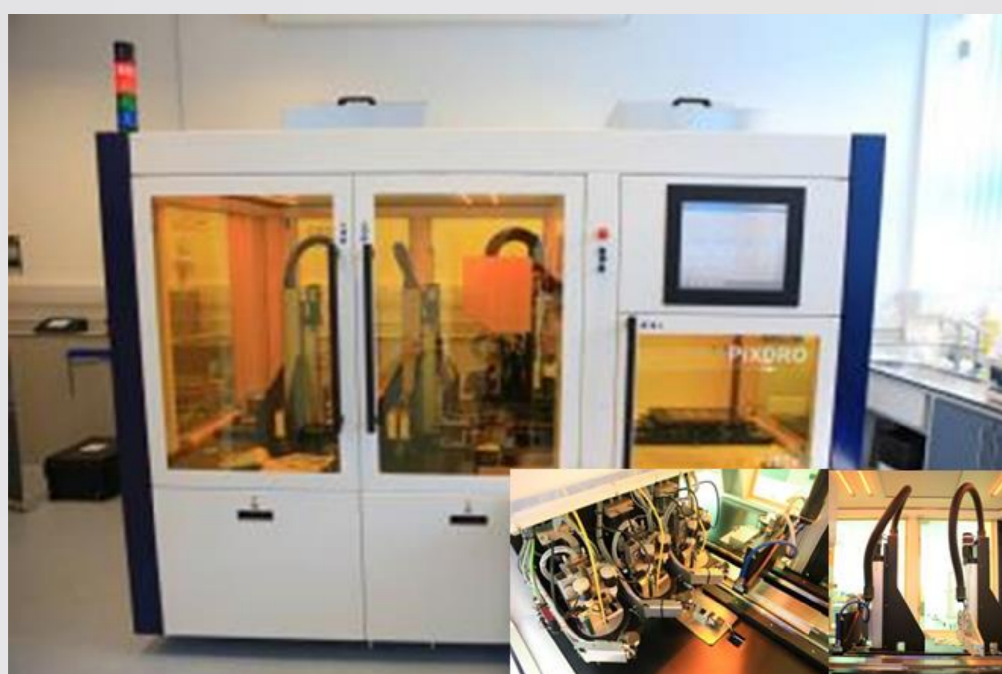
JETx® inkjet printing system (six head); print head assemblies and infra-red and ultra-violet curing source
