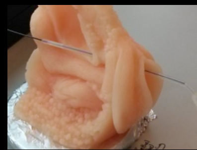
Simulated used testing-insertion force testing using anatomical model
