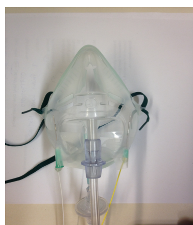
Figure 1: Measuring fibre integrated in nasal cannulae and a CO 2 mask
